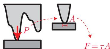
**Figure 2.** An asperity's height determines its area of contact and hence a block's maximum friction force.
