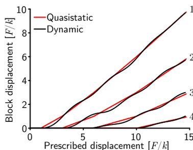
**Figure 3.** Consecutive slip of four blocks with only nearest-neighbor interaction and identical friction forces.
