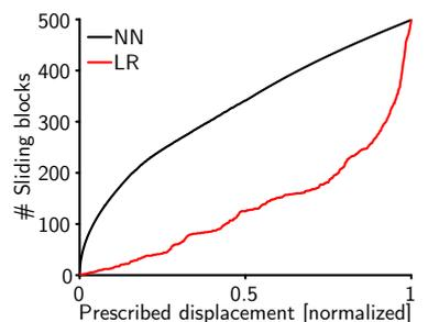
**Figure 5.** Consecutive slip of 500 blocks when the distribution of friction forces is determined by the asperity heights.
