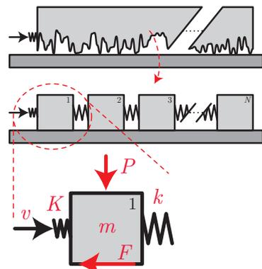
**Figure 1.** Schematic of the computational model. Only nearest-neighbor springs are illustrated.
