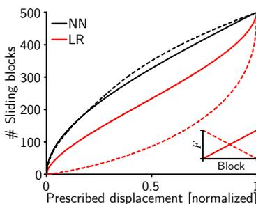
**Figure 4.** Maximum friction forces linearly increasing (solid lines) or decreasing (dashed lines).
